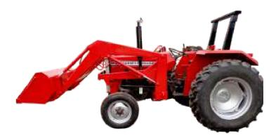
machine for loading stone, brick crush, garbage, sand, grains etc. Hydraulically operated
